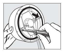
Use a thin screwdriver to remove the two rubber stoppers.
